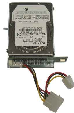
ADAPTER BOARD AND POWER CABLE ATTACHED TO HARD DRIVE (ECS MOTHERBOARDS ONLY)
