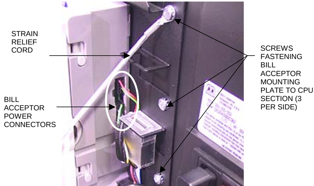
FIGURE 2 - REAR VIEW OF BILLACCEPTOR MOUNTING PLATE
